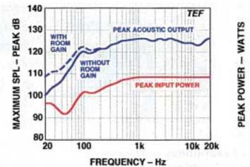
Fig. 9—Maximum peak input power and sound output.
