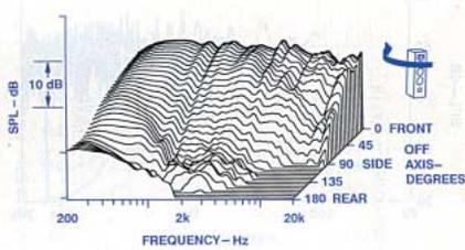
Fig. 3—Horizontal off-axis frequency response.
