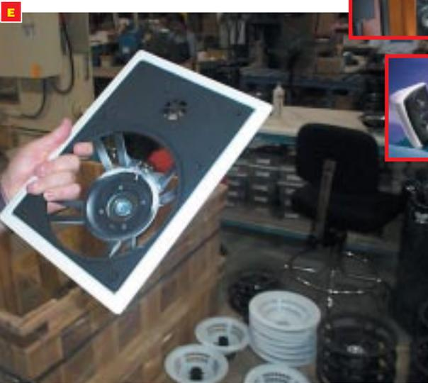
**E. The super-tough plastic chassis for the AMS-100R in-wall speaker is made from an in-house mold.**
