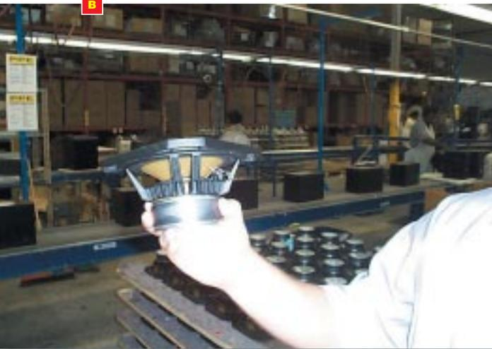
**B. Air holes in the Studio/20's former ventilate the voice coil, which results in reduced distortion and better power handling.**
